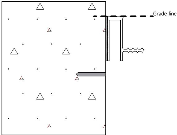
4) Embed prefabricated retrofit waterstop into strip of uncured epoxy.
