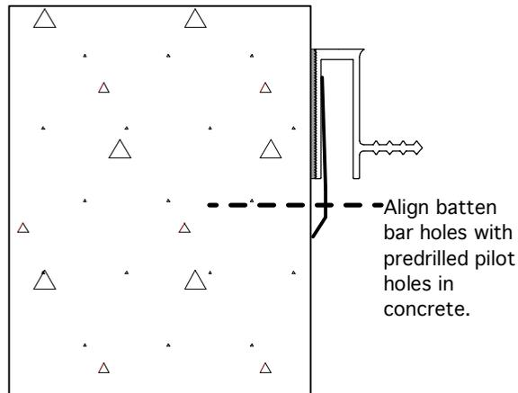
5) Ensure retrofit waterstop is located at the proper grade and position batten bar.
