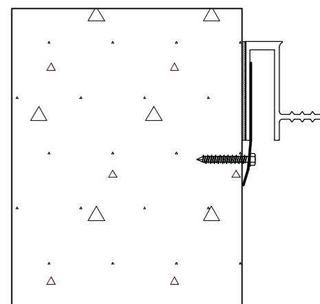
6) Install fasteners through washer, batten bar and into the predrilled pilot holes in the concrete. Tighten fasteners using CONDRIVE® 1000 by ITW Ramset/Red Head until completely seated. (Clutch mechanism in CONDRIVE protects the Tapcon anchor from over-tightening. The stainless steel batten bar will compress as fastener is tightened.)
